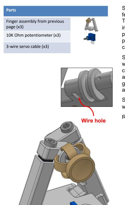
Strip one end of the cables (leaving a female connector on the other end). Thread the cable through the hole in p5 indicated below (with the stripped leads pointing upwards) and then thread a piece of heat shrink tubing over the cable.
