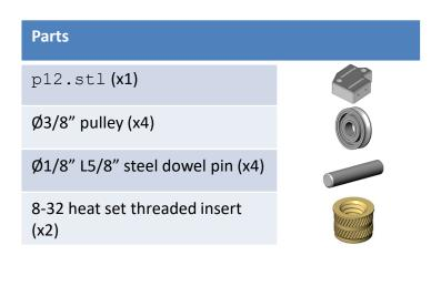
Install the heat press insert into the bottom of p12 with a soldering iron.
