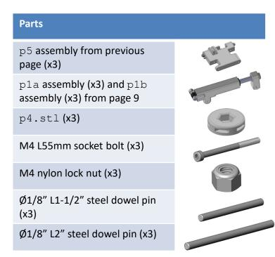
Attach two actuator assemblies to each copy of the p5 assembly using the dowel pins as pictured below.
