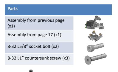
Secure the p12 assembly to w1 with the socket bolts (note, the fingers are excluded in the figure for clarity).
