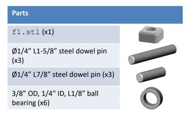
Use f1 as a fixture to press-fit the ball bearings onto the dowel pins. Use an arbor press, a vice, or a hammer to install the pins. Be sure to not damage the bearings. The fixture will ensure that the bearing spacing is correct.
