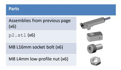
Screw together each p2 component with an actuator assembly using the M8 bolt and nut. Do not over-tighten the bolt, as it can damage the actuator.
